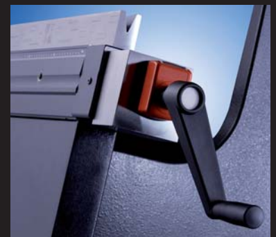
Manually operated with "H" hand crank assembly
