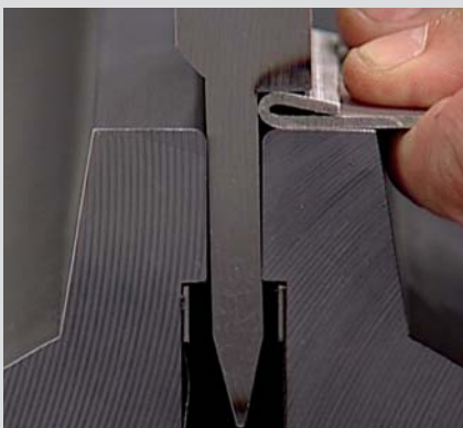
Pre-bend and flattening in the same tool.
