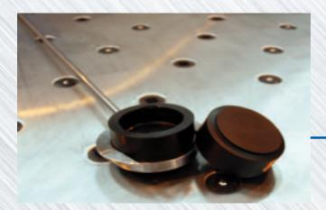
This essentially reduces set-up time between jobs and also eliminates the need for the cumbersome manual method of punching the strippers whilst in the machine.
